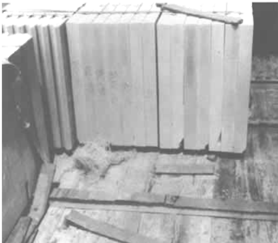
Chipped stones may be useable. Will the chips cover? Are they on the back? Can the stone be cut down and used elsewhere?
