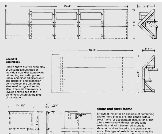
need for masonry back-up. By utilizing the strength of the steel it allows reduced thicknesses and sizes of stone panels, thereby reducing weight and cost.
