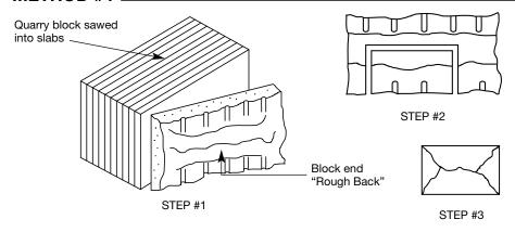
STEP #1—When sawing a quarry block into slabs the block end "rough back" can be used to fabricate a piece of rock face.
