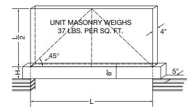
The Beam & Lintel Table is based on a rectangular loading pattern as shown. The actual loading by unit masonry when mortar sets approximates a triangle as shown by the dotted lines. Therefore, the table is conservative.
