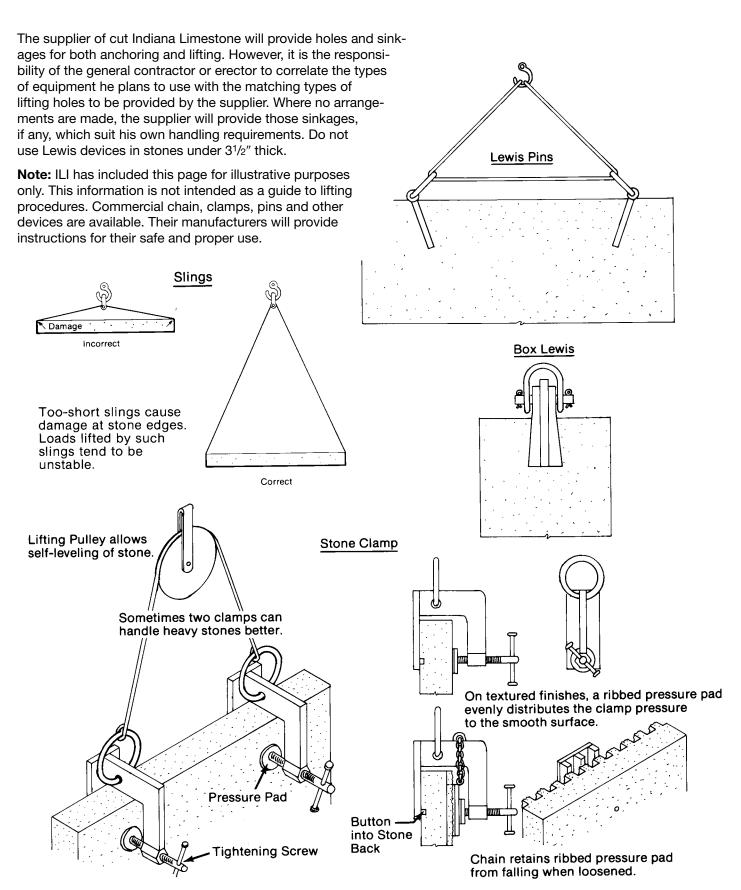
Note: Pins, box Lewises and other devices attached to or near the tops of stones should not be used to raise stone panels to vertical position from the horizontal. They may, however, be used in conjunction with slings or other devices which support the main weight of panels while turning them to the position for installation. In contemporary stone design and usage, Lewis devices are unreliable and dangerous. ILI recommends against their use by persons unfamiliar with safe practices.
