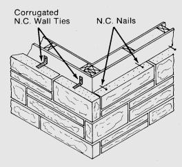
Stone Veneer Anchored to Wood Frame Backing
