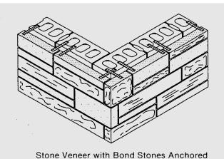
to Concrete Block Backing.
