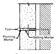
Tool the pointing mortar to compact the joint.
