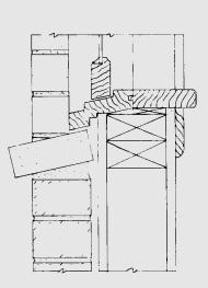
Flat sawed-stone sills may be tipped for wash surface, or set flat in windows or as capping for wing-wall extensions. This is particularly effective when used as band course at sill level. Dealer or his supplier can provide specially sawed shapes where checked-out areas are needed.
