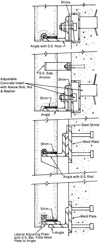
**Note:** The preferred location of gravity shelves is in the bottom bed or at least in the bottom 1/3 of the panel.
